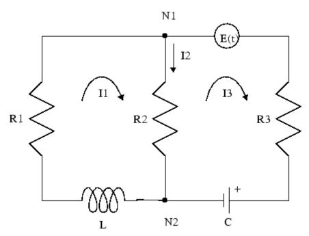
Let Rj and Ij, j = 1, 2, 3 be resistances (measured in ohms) and currents (amperes), respectively; L be inductance (henrys), and C be capacitance (farads); E(t) be the electromotive force, and Q(t) be the charge.
