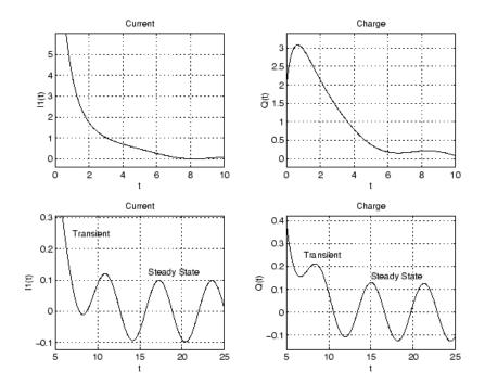
Note that the circuit's behavior, which appears to be exponential decay in the short term, turns out to be oscillatory in the long term. The apparent discrepancy arises because the circuit's behavior actually has two components: an exponential part that decays rapidly (the "transient" component) and an oscillatory part that persists (the "steady-state" component).
